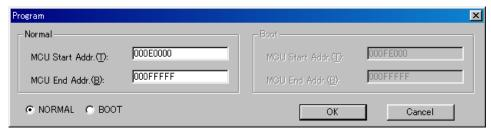
Fig. 9.1: Parameter Input Dialogue of Program Command
